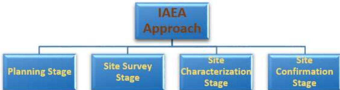
Fig. 1 Flowchart of a Systematic approach for site selection of NPPs.(After IAEA,1994)
